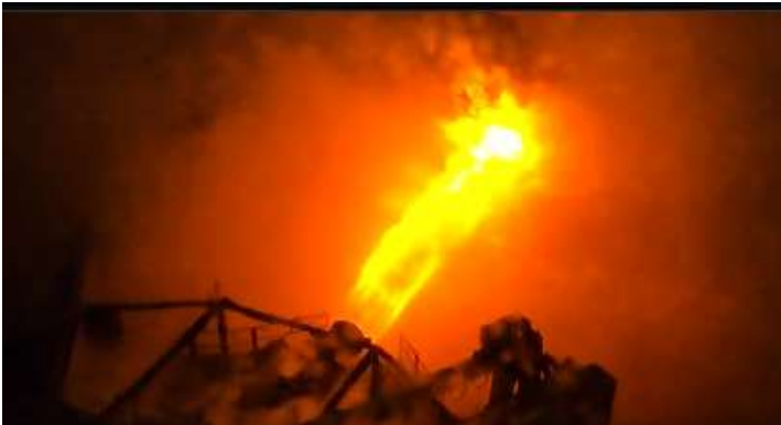
SpaceX Raptor Engine Fires Into Water Cooled Steel Plate. SpaceX Image.
