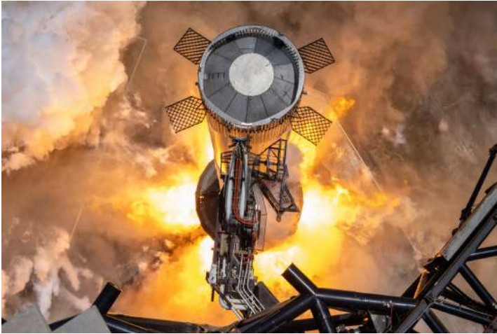
Static Fire Test of Booster 9, August 28. SpaceX
