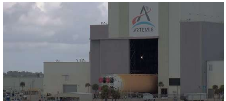
SLS Core Stage Enters VAB Transfer Aisle at South End of VAB. NASA image.
