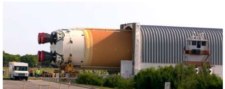
SLS Core Stage Emerges from the Pegasus Rocket Transport Barge. NASA Image.
