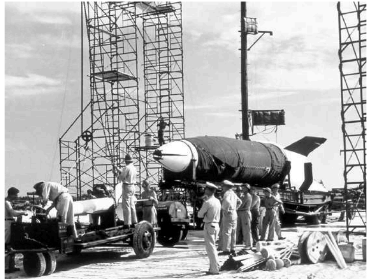
The Bumper 8 Rocket is Prepared for Launch. Cape Canaveral, July 1950. The V-2 at right is being prepared to receive the WAC Corporal rocket on the cart at left. NOAA image.
