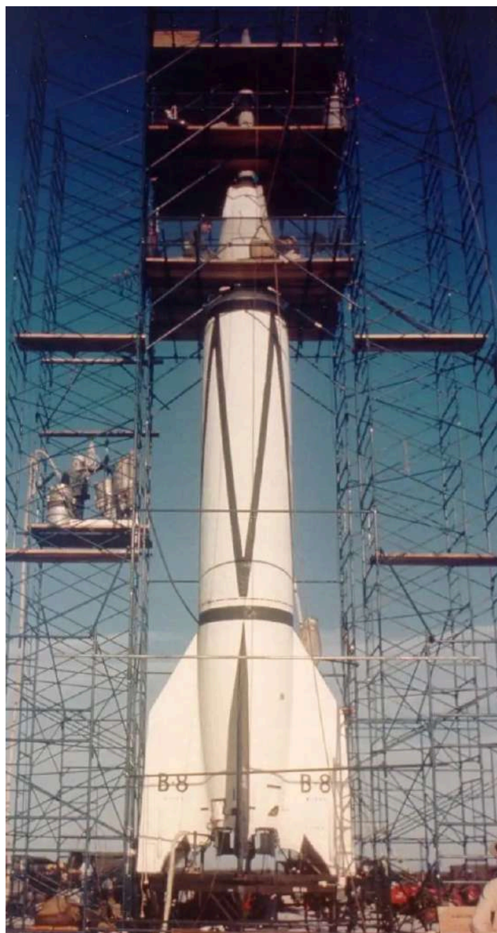
Bumper 8 in its gantry during launch preparations in July 1950. Note the “B8” designation on its fins. NASA photo.
