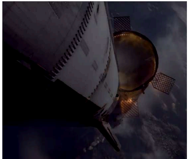
Hot Staging of the Ship from the Booster. A blocked section of the hot staging ring helps direct the Booster in its flip prior to boosting back toward the Texas coast, saving propellant versus a random flip direction. SpaceX image.
