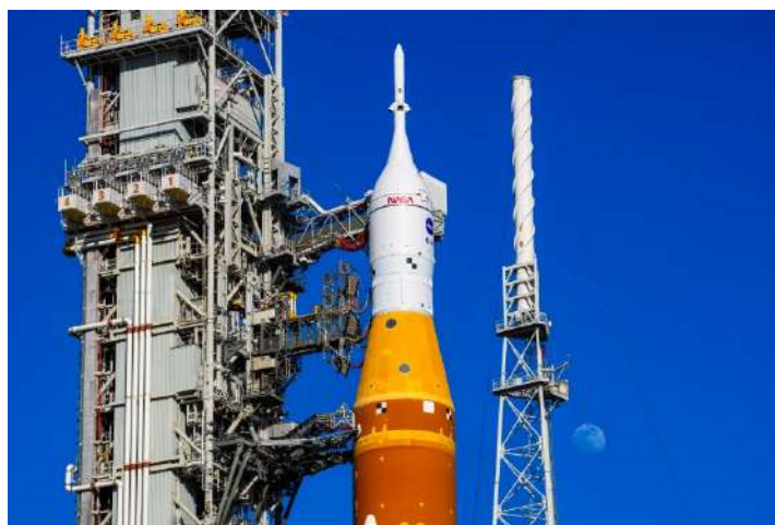
Moon Rising Behind Artemis II prior to rollback. The access hatches are visible as two gray circles in the light orange cone below the capsule and service module in white. NASA image.
