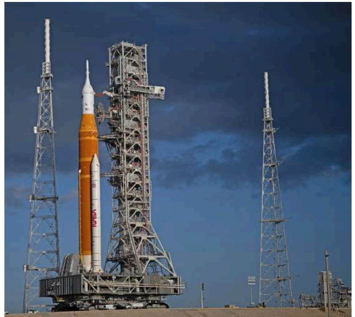
The crawler-transporter returns the SLS and its mobile launch platform to LC-39B on March 20th, following repairs at the VAB. NASA image.
